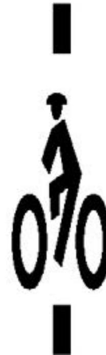
**Marking indicating to wait at the middle of the lane in newer, quadrupole installations.**
